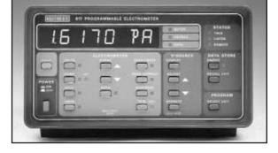
In addition to standard resistance functions using constant current, the 617's variable voltage source can supply from 50mV to 102V, which can be applied to a resistance and the resulting current or resistance displayed.
